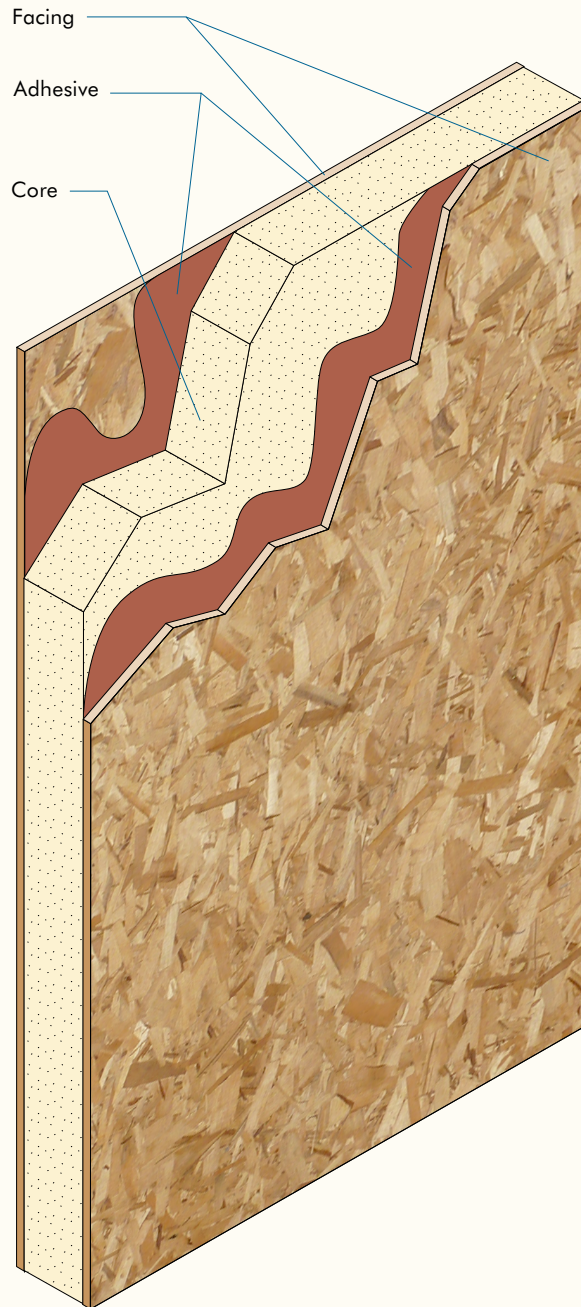
EXAMPLE OF A SIP WALL PANEL (for foamed-in-place foam cores, the foam is the adhesive)
